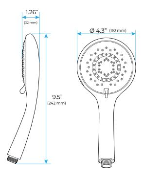
Flow Rate: 2.0 GPM / 7.6 LPM
